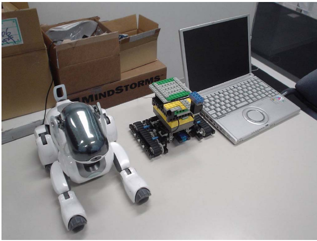
Fig. 2. Three robots utilized in this experiment: AIBO, Mindstorms, and PC (from left to right).
